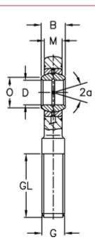
$\begin{array}{lll} A & = 160 \\ a \ (degrees) & = 6 \\ B & = 49 \\ D & = 70 \\ Dynamic \ drive \ (kN) = 315 \\ F & = 235 \\ g & = M56x4 \\ GL & = 125 \\ \end{array}$
